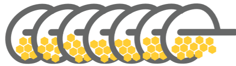
Transportation using augers
